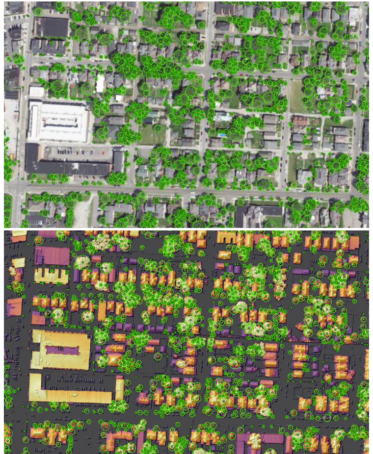
Figure 3: Locations of individual trees and their crowns derived from the 2019 LiDAR, overlaid on 2021 aerial imagery (top), and the 2019 LiDAR map (bottom).
